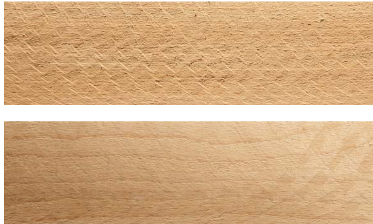
Fig. 4: The direct comparison shows the high-precision glue-line cut achieved on a machine of the Q series (bottom).
