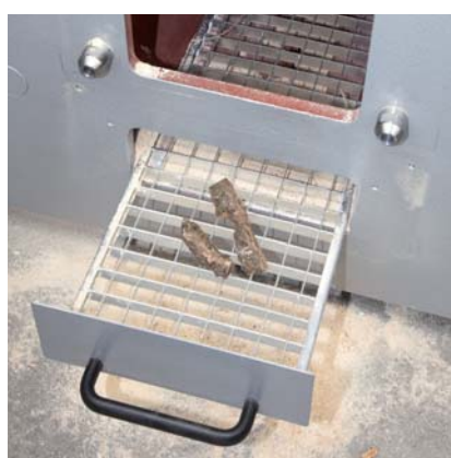
Fig. 2: A grate (option) prevents large splinters and wane sections from getting into the dust extraction system.
