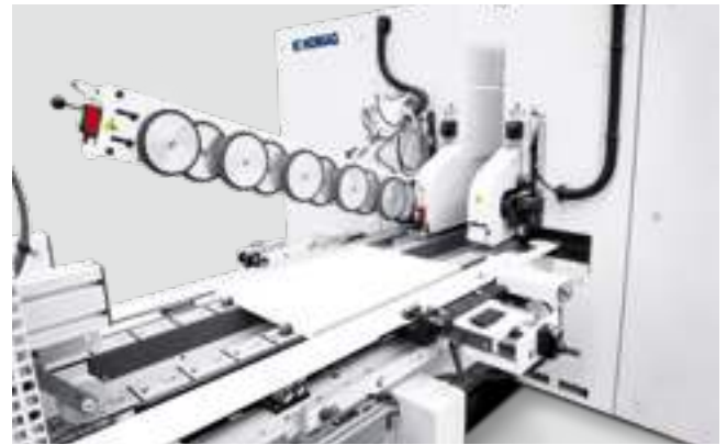
Transverse processing with EDGETEQ D-810 powerLine The steplessly adjustable cams of the transport chain form the workpiece stop. This allows even softforming parts or profiled components to be reliably transported through the machine without damage.
